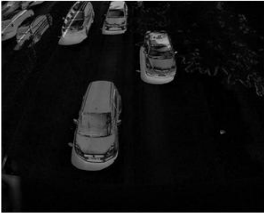
Figure 4. The result of background subtracting in between frames
