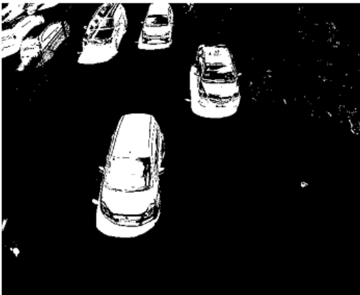
Figure 5. The binary image of Otsu Thresholding
