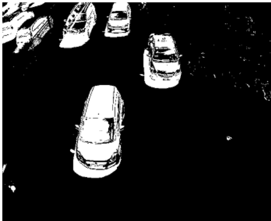
Figure 5. The binary image of Otsu Thresholding
